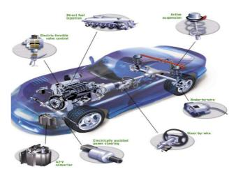
Figure 5: Mechatronic Systems in Automobile
