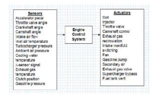
Figure 11: Mechatronic Elements of Engine Control System
