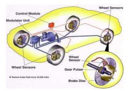
Figure 7: Antilock Brake System (ABS)
