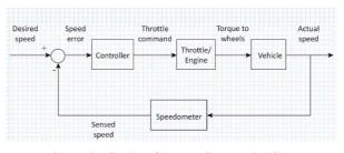
Figure 9: Cruise Control System in Car
